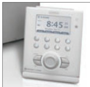
*The removable control panel serves as a remote control. Bidirectional communication allows the panel to show the contents of your iPod, the tune you've selected, etc.*
